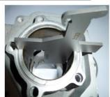
In this position the template may not touch the cylinder wall.
